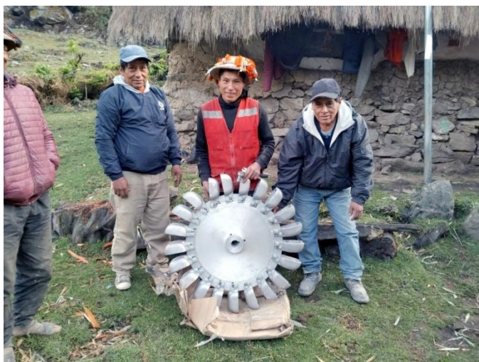
The Pelton turbine with the impeller blades converts the kinetic energy of the water into electricity.
